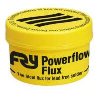
Powerflow Flux is a soft, white paste which is easily applied to jointing areas prior to soldering. It is designed for the soldering of copper plumbing systems and is suitable for use with a wide range of metals and alloys. It contains no zinc oxide.
