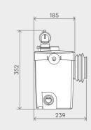
Discharge Pipework 22 / 28 / 32mm
