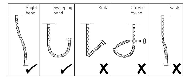
**Important:** Failure to follow these guidelines may result in poor performance and damage to the flexible connection hose.
