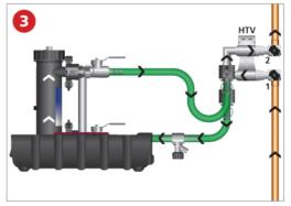
Having completed the installation of the MagnaClean, remove the filter and attach the MagnaCleanse hoses between the RapidFlush Filter and the MagnaCleanse HTV connector attached to the isolation valve on the pipework.
