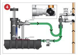
Turn OFF isolation valves on the RapidFlush Filter. Loosen and remove the lid assembly from one of the RapidFlush Filter canisters.
