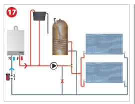
Top up the system allowing the header tank to fill to the required level. Once complete, remove drained MagnaCleanse assembly, disconnect and reinstall MagnaClean filter to the isolation valves. If this method is not appropriate ensure a full drain down is carried out.
