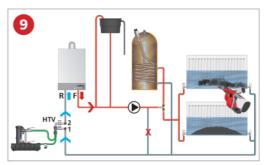
Continue the VibraClean radiator agitator to dislodge any sludge deposits until the return hose to the RapidFlush Filter runs clear.
