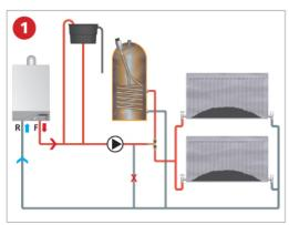
Identify the three port valve and confirm manual operation. If not, install an isolation valve on the cylinder flow or return. Complete all relevant preliminary electrical safety checks to boiler and pipework confirming safe isolation and earth path, isolate central heating system and drain.
