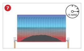
Turn on heating system (all radiators open) for 15 minutes. The radiators should be hot at the bottom, cold at the top.
