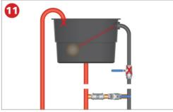
Set the boiler control to OFF. Attach a drain hose to the MagnaCleanse drain valve and secure with a jubilee clip. Temporarily cap off the expansion pipe. Temporarily connect the cold mains supply and tank cold feed supply (to bypass header tank) including a combined stop tap and pressure gauge to control the water pressure.
