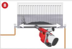
Turn OFF the hot water circuit, by-pass valves and all the radiators, leaving only one radiator open at a time. With the system running, using ADEY's VibraClean tool attached to an SDS drill, set to hammer only mode with no rotary action and agitate each radiator for 15-20 seconds.
