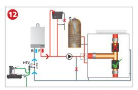
Turn OFF the HTV isolation valve 2. Open the heating circuit only (two or three port valve) leaving the cylinder flow closed. Check all radiators and bypass are turned off, leaving the furthest radiator from the boiler open.
