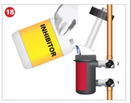
Add a recommended inhibitor into the canister i.e. use the pro-fill bleed valve or remove canister lid assembly and pour into the filter (holds approximately half a litre). Open up the isolation valves and remove any air.
