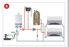
Re-fill and pressurise the central heating system ensuring the radiators are half-full. Check for leaks.
