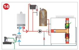
When complete fill and vent the radiator and allow to circulate for 30 seconds. Repeat this process on each radiator until complete. Always open up the next radiator, before turning off the cleansed radiator. Once all radiators have been cleansed, open the domestic hot water port, then close the central heating port. This flushes the indirect coil inside the cylinder.
