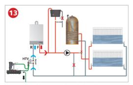
Turn on the cold mains supply and allow the mains water to flush through the pipework, partially filled radiator and return. Allow the water to drain out to a convenient point outside until clear.
