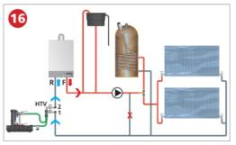
Once complete, turn OFF the HTV isolation valve 2 and the cold mains supply. All the radiators should be full and valves open. Remove the header tank and thoroughly clean. Reconnect. Remove the cap from the expansion pipe and reconnect the cold mains supply to the header tank supply and the cold feed system supply.
