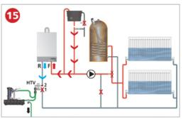
Having completed the previous step, turn ON the HTV isolation valve 2 on the return to the boiler and turn OFF the HTV isolation valve 1 from the system, close the DHW port and allow the cold water to flush through the boiler and RapidFlush filter.
