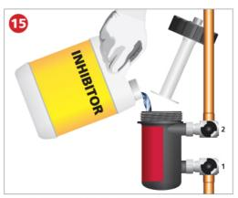
Add a suitable inhibitor into the canister i.e. use the Pro-Fill bleed valve or remove canister lid assembly and pour into the filter (holds approximately half a litre). Open up the isolation valves and remove any air.
