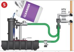
Add a suitable cleanser to the system via the RapidFlush Filter canisters.
