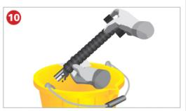
Isolate and clean the RapidFlush Filter as required. Using Personal Protective Equipment i.e. gloves and paper towels, wipe off any magnetite into a bucket or waste bag and dispose of correctly. When satisfied, open up the next radiator, turn off the treated radiator and repeat the process until all radiators are clean.
