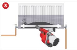
Turn off any by-pass valves and all the radiators, leaving only one radiator open at a time. With the system running, using ADEY's VibraClean tool attached to an SDS drill, set to hammer only mode with no rotary action, agitate each radiator for 15-20 seconds.
