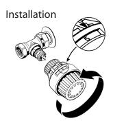
Remove the valve cover. Check that the thermostat is set at the factory setting of 5.
