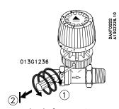
To remove the theft protection use screwdriver 013G1236 and screw into the hole (1). Pulled out until the stop is reached (2).
