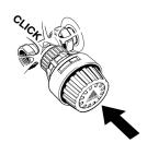
Push the thermostat firmly onto the valve until an audible "click" is heard.
