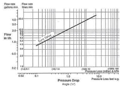
**LOCKSHIELD WITH DRAIN OFF FACILITY FOR BOTH MATCHMATE AND EUROVALVE**
