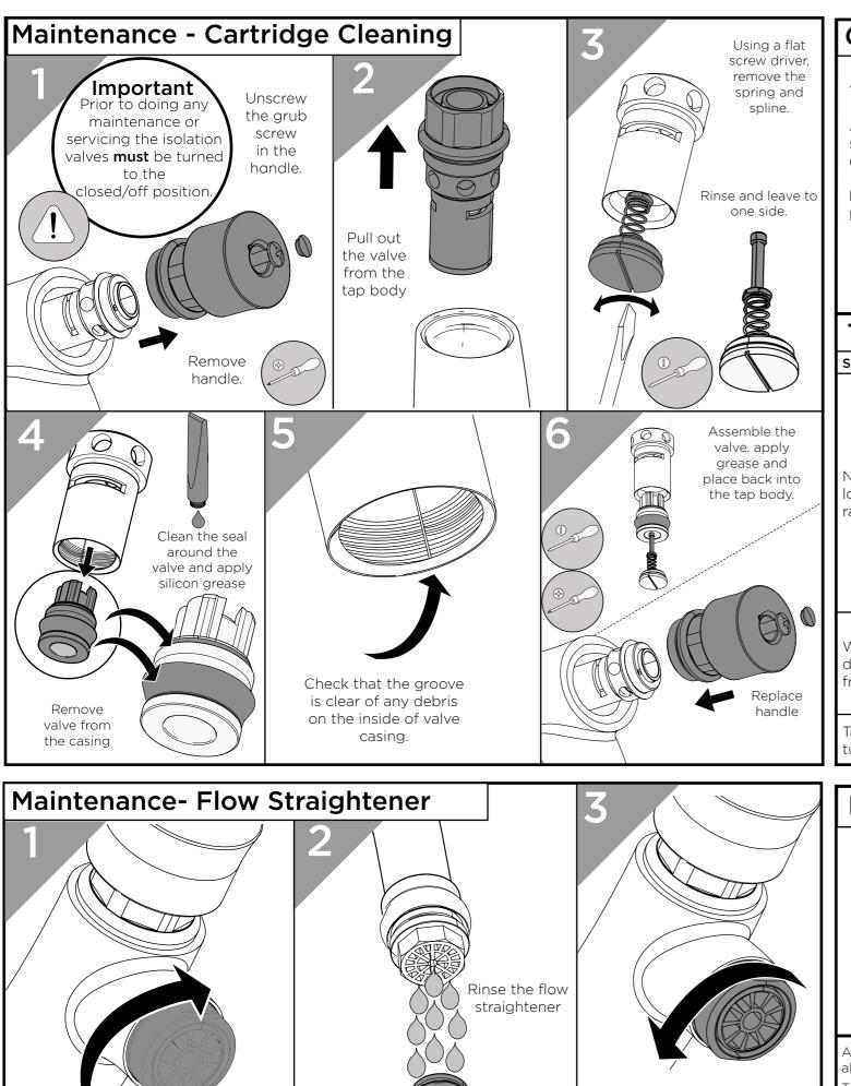
Replace flow straightener into spout.
