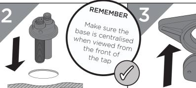
Feed the Reinforcing Plate, (if required) and Back nut up to the underside of the sink.
