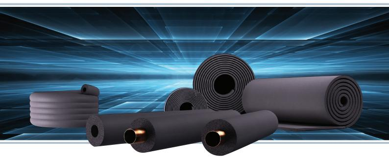
Flexible closed cell rubber insulation, Kaiflex ST Class 0 reliably prevents condensation and reduces energy loss. By incorporating a water vapour barrier into the insulation cell structure Kaiflex ST Class 0 can effectively eliminate water vapour migration and retain outstanding performance over the entire system life.
