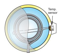
Temperature sensor is supplied with unit. Fit as shown (see also 'Electrical installation').
