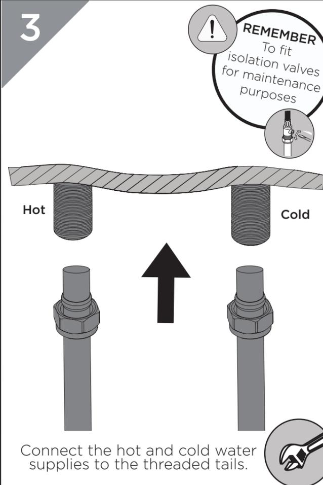
Connect the hot and cold water supplies to the threaded tails.
