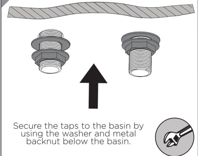
Secure the taps to the basin by using the washer and metal backnut below the basin.
