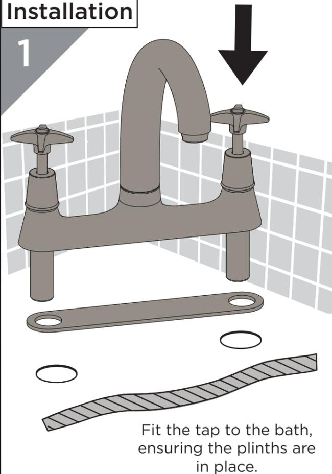
Fit the tap to the bath, ensuring the plinths are in place.
