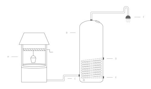
A - Well B - Well Wizard C - Cold flow from well D - Coil flow
