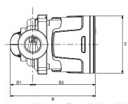
Maximum Flow: 60 Litres/Minute Maximum working head: 6.7 Metres Maximum closed valve head: 6.9 Metres
