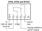
Note: Link between terminals L and 1 if mains voltage is required on the thermostat switch.
